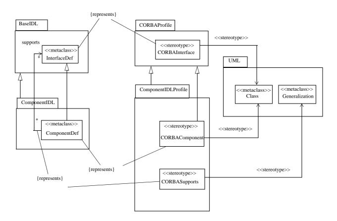
Figure 8.10 - Component mapping
