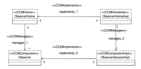
Figure 9.14 - The Composition model for the Observer component
