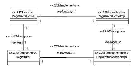
Figure 9.13 - The Composition model for the Registrator component
