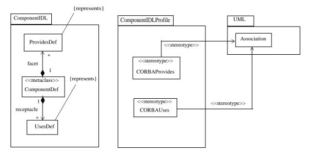
Figure 8.11 - Ports mapping
