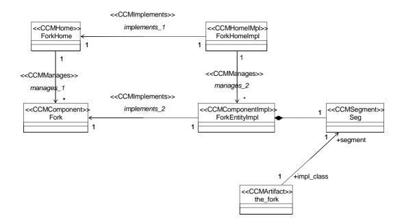
Figure 9.12 - The Composition model for the ForkComponent
