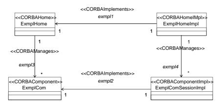
Figure 8.17 - CIDL composition: unit of a component implementation in CCM
