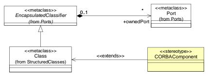
Figure 8.21 - ComponentIDL Profile: Extended UML classes (I)
