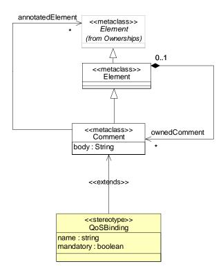
Figure 8.30 - CCMQoS Profile: extended UML classes
