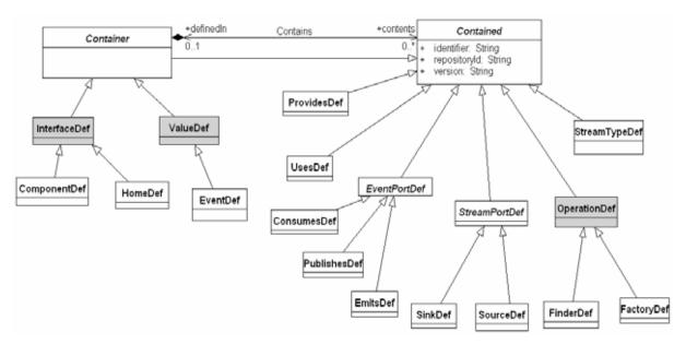
Figure 7.6 - ComponentIDL Containment hierarchy
