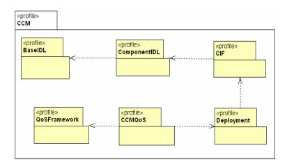
Figure 8.1 - CCM Profile package structure
