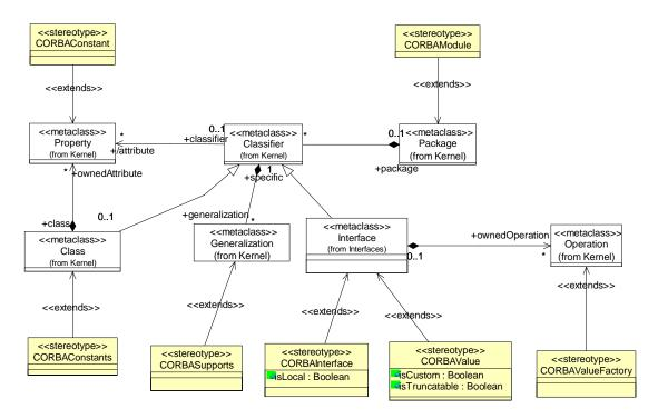
Figure 8.2 - BaseIDL Profile: Extended UML classes (I)
