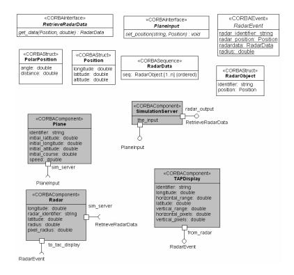
Figure 9.2 - User-defined data types, interfaces and components
