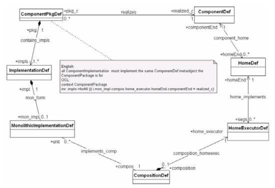
Figure 7.10 - Component package and Implementations
