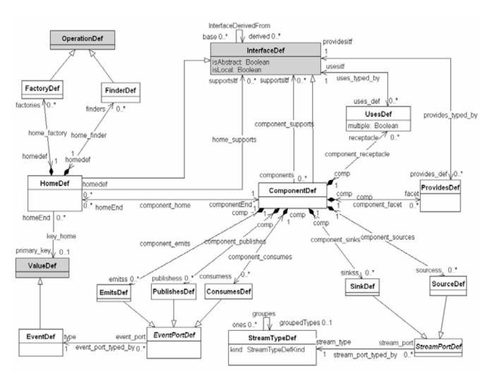
Figure 7.4 - ComponentIDL Metamodel
