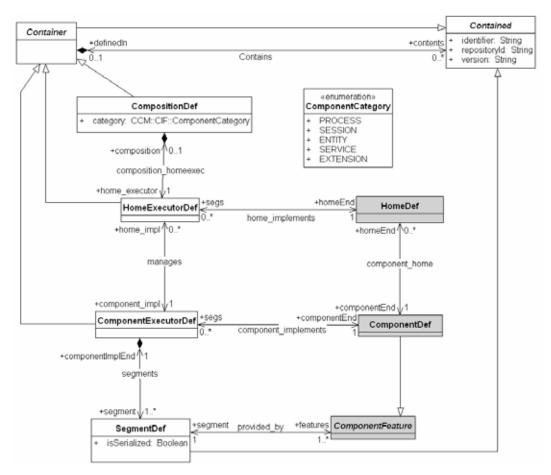
Figure 7.8 - Component Implementation Framework Metamodel
