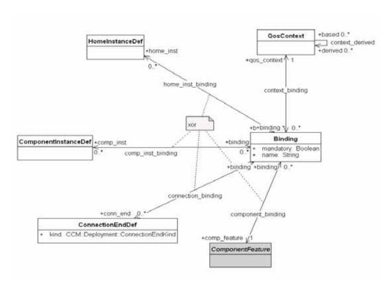
Figure 7.17 - CCMQoS metamodel: Binding
