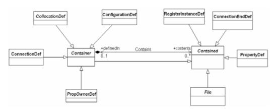
Figure 7.15 - Deployment and Configuration containment
