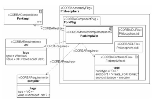
Figure 8.28 - Deployment Profile example: package structure of an application
