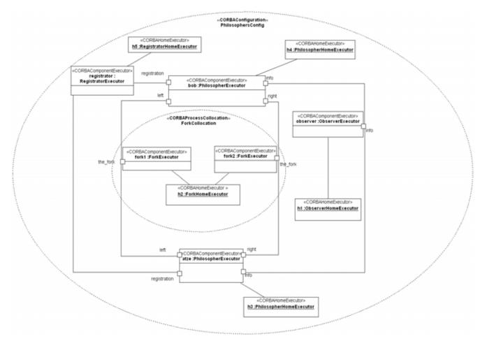
Figure 8.29 - Deployment Profile example: initial configuration of an application
