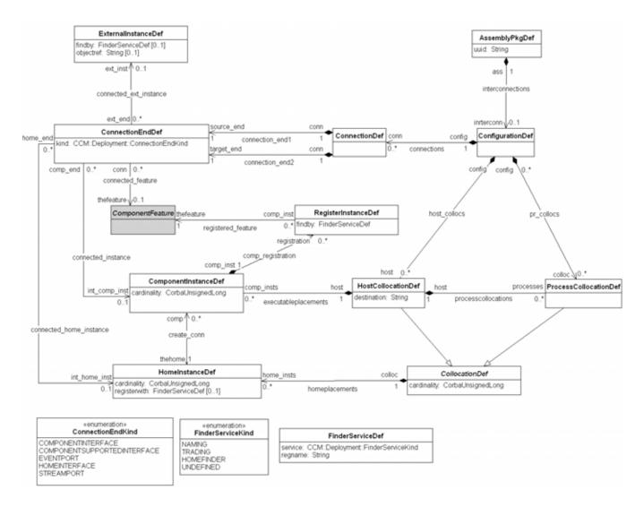
Figure 7.12 - Assembly package description
