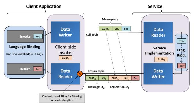
Figure 7.1 - Conceptual View of Remote Procedure Call over DDS
