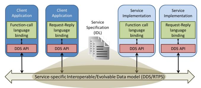
Figure 7.2 - Strong decoupling of language binding (function-call and request /reply) from the service-specific data model
